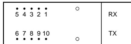
Figure 1. 1417K4A Transceiver, 10-Pin Configuration, Top View
