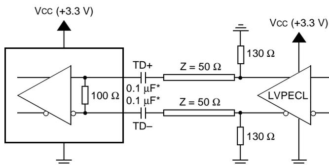
\* OPTIONAL ac COUPLING CAPACITORS; USE CERAMIC X7R OR EQUIVALENT
