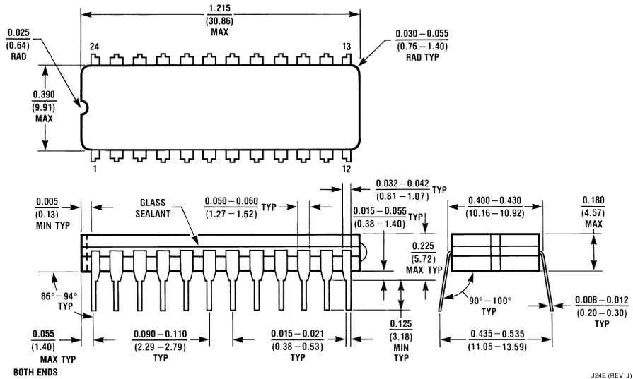
**24-Lead Ceramic Dual-In-Line Package (0.400" Wide) (D)**
