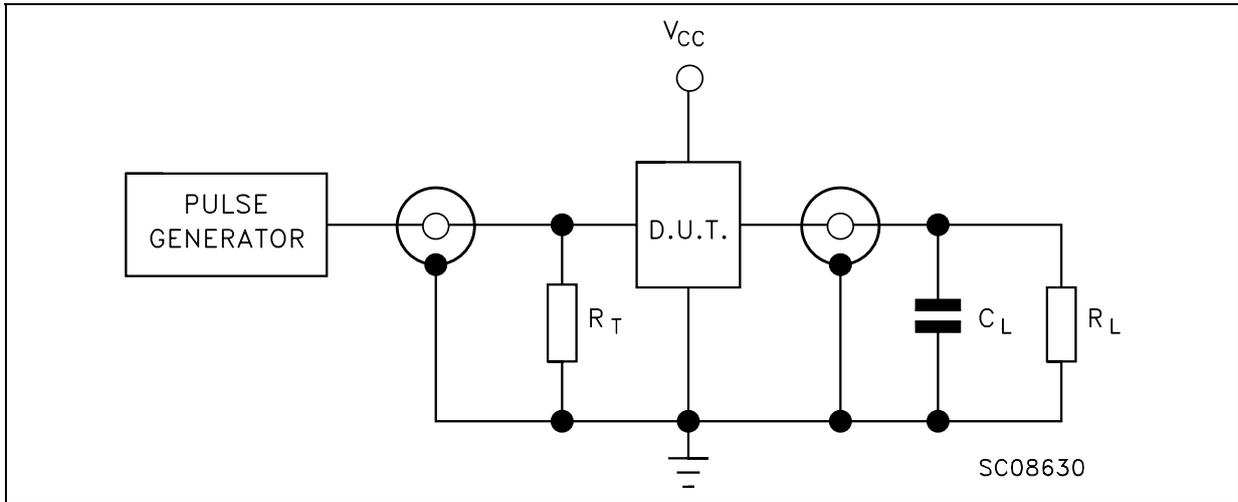
$R_T = Z_{OUT}$  of pulse generator (typically 50Ω)
