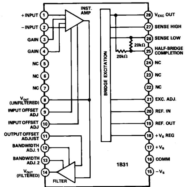
pair of thin-film 20k $\Omega$  resistors is connected across the excitation outputs. This assures temperature tracking of  $\pm 5\text{ppm}/^\circ\text{C}$  max and reduces part count.
