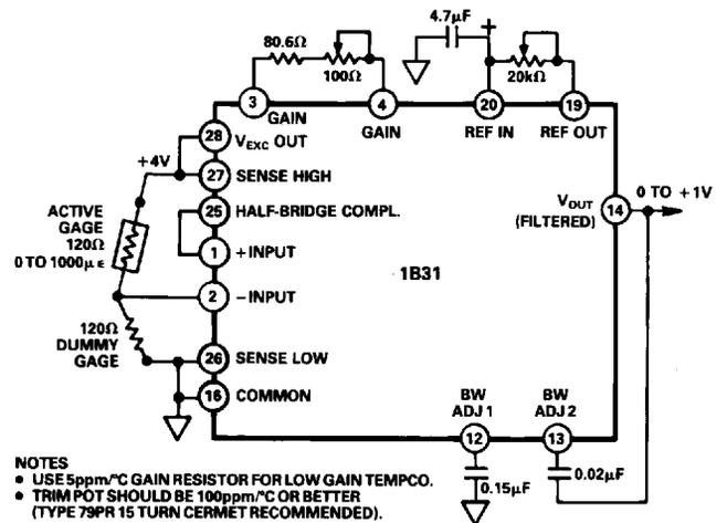
Figure 15. Strain Gage Application Using Internal Half-Bridge
