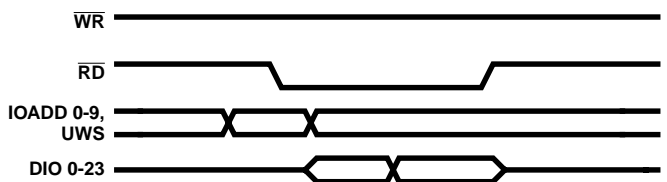
FIGURE 15. ASYNCHRONOUS 16/24 MODE TIMING
