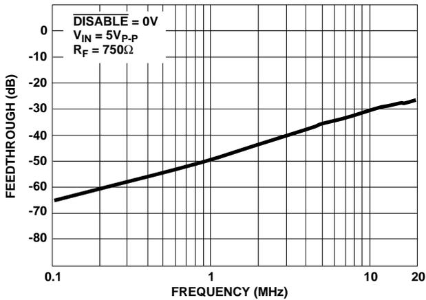
FIGURE 33. DISABLE FEEDTHROUGH vs FREQUENCY
