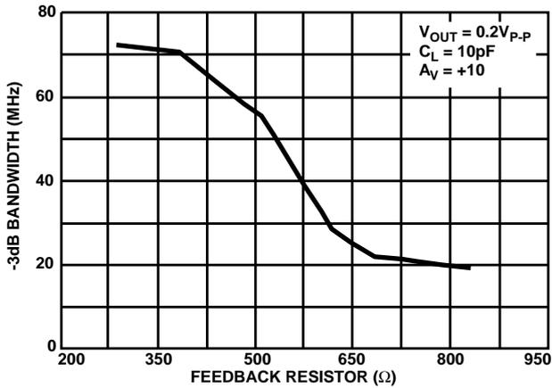
FIGURE 7. BANDWIDTH vs FEEDBACK RESISTANCE
