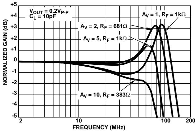
FIGURE 1. NON-INVERTING FREQUENCY RESPONSE
