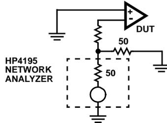
FIGURE 2. TEST CIRCUIT FOR TRANSIMPEDANCE MEASUREMENTS
