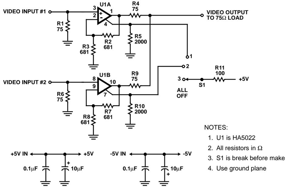
FIGURE 39. TWO CHANNEL HIGH IMPEDANCE MULTIPLEXER
