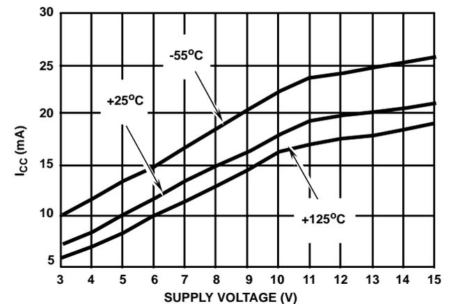
FIGURE 30. DISABLE SUPPLY CURRENT vs SUPPLY VOLTAGE
