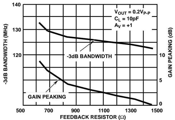
FIGURE 4. BANDWIDTH AND GAIN PEAKING vs FEEDBACK RESISTANCE
