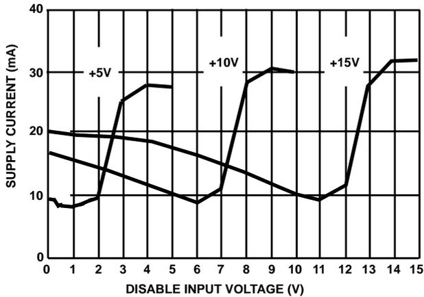
FIGURE 25. SUPPLY CURRENT vs DISABLE INPUT VOLTAGE
