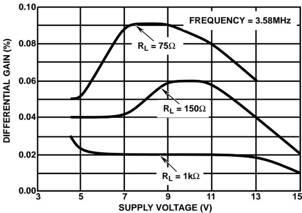
FIGURE 9. DIFFERENTIAL GAIN vs SUPPLY VOLTAGE
