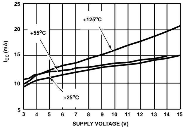
FIGURE 23. SUPPLY CURRENT vs SUPPLY VOLTAGE
