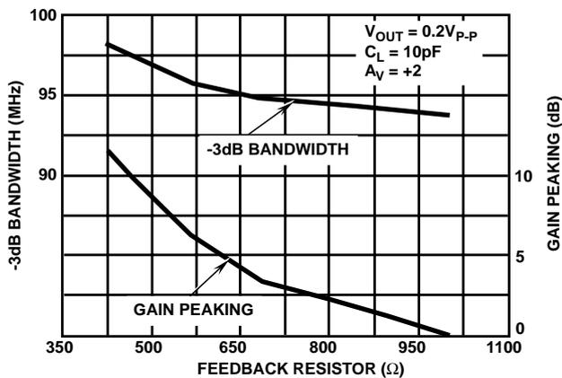
FIGURE 5. BANDWIDTH AND GAIN PEAKING vs FEEDBACK RESISTANCE
