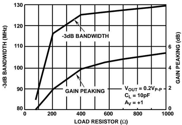
FIGURE 6. BANDWIDTH AND GAIN PEAKING vs LOAD RESISTANCE
