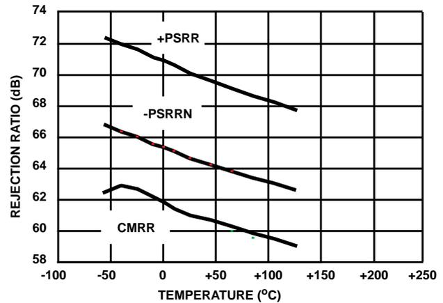
FIGURE 24. REJECTION RATIO vs TEMPERATURE
