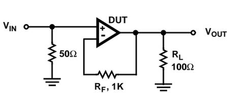
FIGURE 3. SMALL SIGNAL PULSE RESPONSE CIRCUIT
