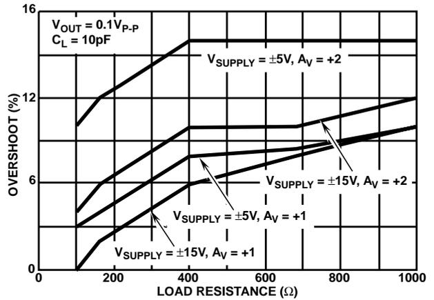
FIGURE 8. SMALL SIGNAL OVERSHOOT vs LOAD RESISTANCE
