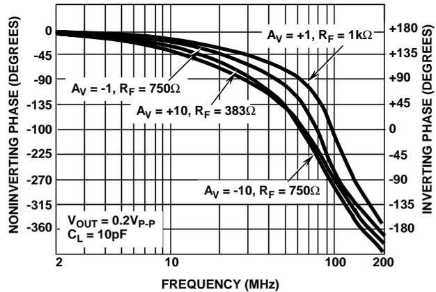
FIGURE 3. PHASE RESPONSE AS A FUNCTION OF FREQUENCY
