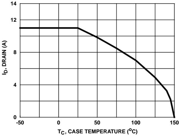
FIGURE 3. MAXIMUM CONTINUOUS DRAIN CURRENT vs TEMPERATURE
