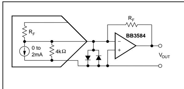
FIGURE 11. External Op Amp Using External Feedback Resistors.
