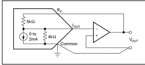
FIGURE 9. External Op Amp Using Internal Feedback Resistors.
